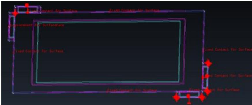
Fig. 3 Single masonry wall modeling and boundary conditions (ATENA)
