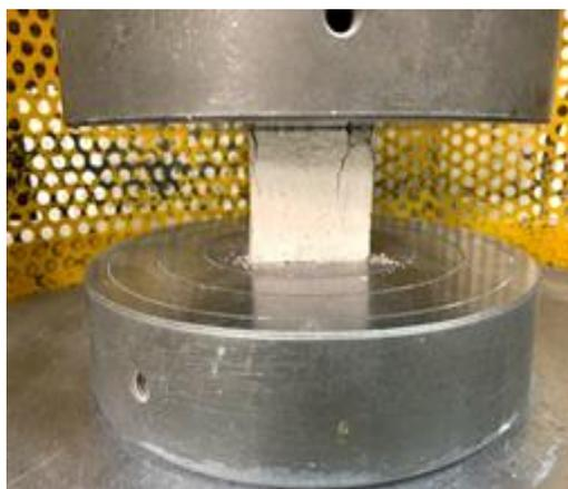
Fig. 2 Mortar compressive strength test
