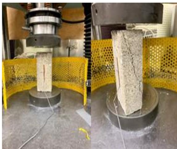
Fig. 1 Concrete brick compressive strength test
